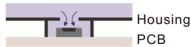
Figure 11: Suitable windows on the enclosure provide good access to environmental measurements and allow for greater air exchange.
